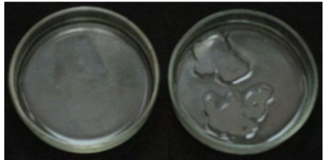
Figure 5. Left: 5 ml of water with negative electric charge cover all the bottom of a Petri dish. Right: 5 ml of water with positive electric charge do not cover the bottom of a Petri dish; the surface of such water decreases rapidly after mixing [13].
