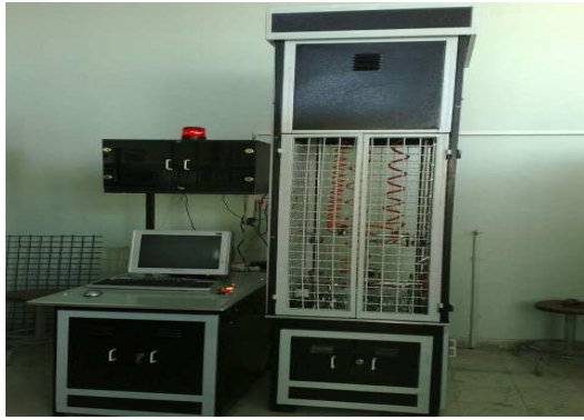
Figure 9. Impact test machine.
