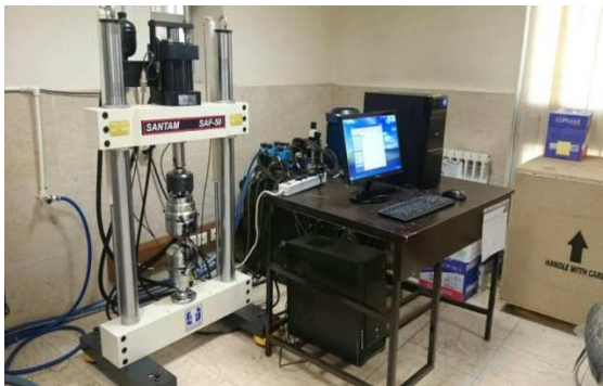
Figure 10. Fatigue test configuration.
