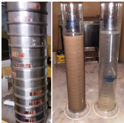
Figure 3. Photograph of the series of sieves and two test specimens.
